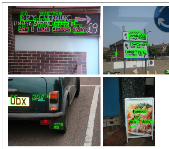
Figure 5. Optical character recognition in real time.
